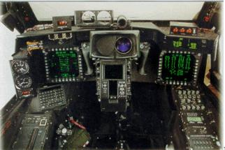
In addition, data were obtained for three other areas: The Co-Pilot Gunner (CPG) instrument panel was a good candidate for DFMA due to its assembly complexity, number of parts and rivets required to assemble it. It included the Up-Front Display (UFD) tray and the Multifunction Display (MFD) tray. These last two sub-assemblies of the CPG instrument panel made it very difficult to assemble and require extensive labor for the assembly activity and the final installation.
