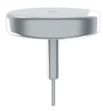
Grasping and manipulating the Piston sub can be done with one hand and no tools, it presents no handling difficulties, and it will not be secured immediately upon insertion into the base. Accept all of the default values in the Handling requirements, Handling difficulties, and Securing process group boxes.
