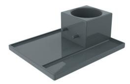
The Plastic base will be acquired by the assembly worker and placed into a simple fixture so that it is ready to receive the remaining parts.
