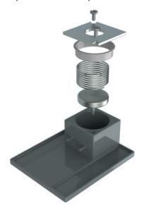
Each of the items pictured will be added to the Structure chart on the left side of the main program window. The DFA questions will then be answered for each item so that the program can estimate the assembly process time and cost.
